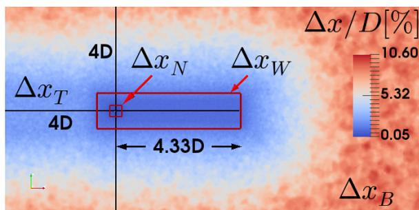
Figure 2: Cell size in the MS2 mesh.  $\Delta x/D[\%]$  is the cell size as a percentage of the turbine diameter. The black lines indicate distances. The hub is contained in the red square. The red parallelepiped delimites the wake refinement area.
