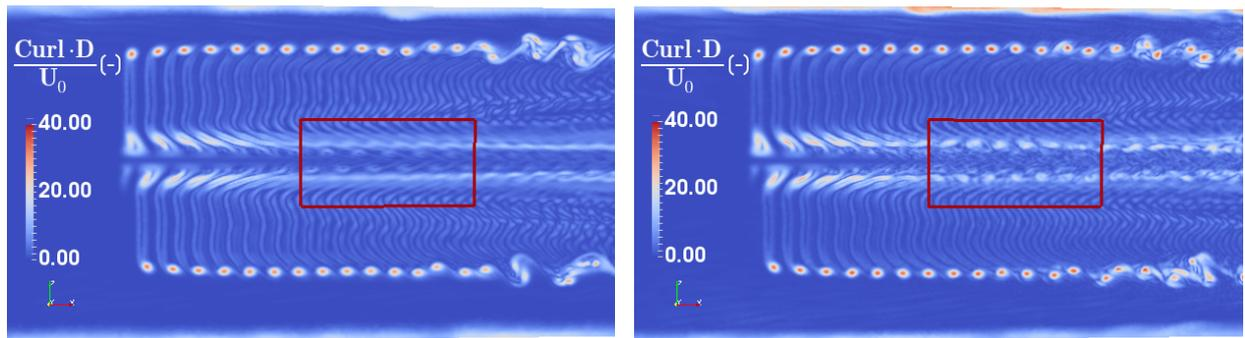
Figure 7: Velocity curl magnitude. Vertical slices of the domain passing by the rotor axis are shown for A2 on the left and for A2\* on the right. The slices were taken at approximately  $t = 17.86$  s. The red square highlights the differences seen at the wake core.
