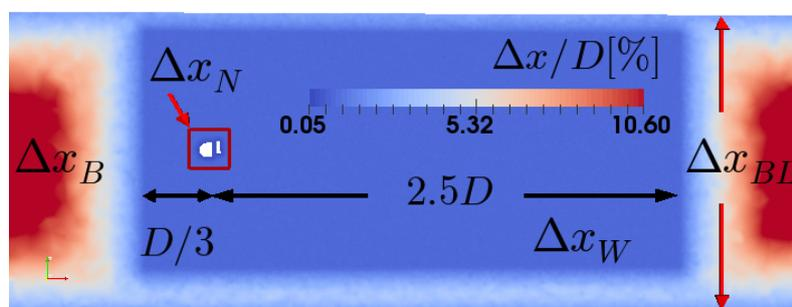
Figure 4: Cell size in the MR2 mesh. The nacelle is at a height of  $0.88D$ . The legend refers to  $\Delta x/D[\%]$ . The two-part nacelle is contained in the red box. The black two-sided arrows indicate horizontal distances.
